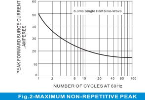
Fig.2-MAXIMUM NON-REPETITIVE PEAK FORWARD SURGE CURRENT
