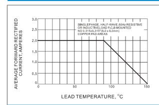
Fig.1 FORWARD CURRENT DERATING CURVE
