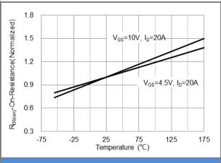
Fig.4 On-Resistance vs. Junction temperature
