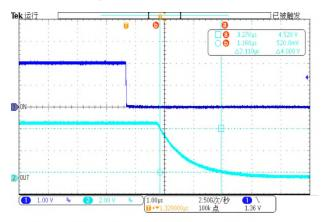
Figure-8. Fall time vs. Input voltage
