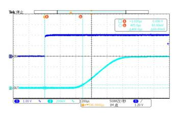
Figure-14. Delay time vs. Input voltage
