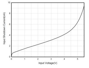
$V_{\text{BIAS}} = 5.5 \text{ V}, V_{\text{ON}} = 0 \text{ V}, V_{\text{OUT}} = 0 \text{ V}$ Figure-4. Input shutdown current vs. Input voltage
