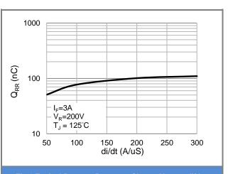
Fig.6 Typical Reverse Recovery Charge Versus di/dt
