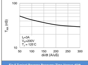
Fig.5 Typical Reverse Recovery Time Versus di/dt
