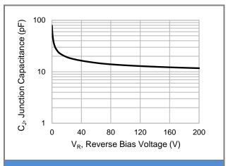
Fig.2 Typical Junction Capacitance
