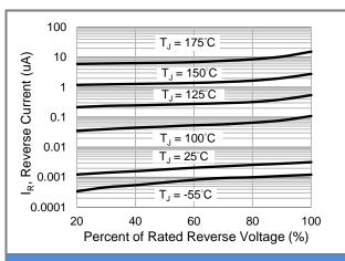
Fig.3 Typical Reverse Characteristics
