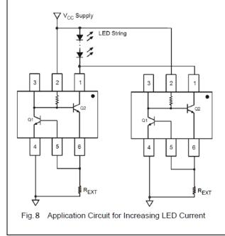
The 2sC164s has been designed for driving low current LEDs with typical LED current of 20mA to 100mA. It provides a cost effective way for driving low current LEDs compared with more complex switching regulator solutions. Furthermore, it reduces the PCB board area of the solution as there is no need for external components like inductors, capacitors and switching diodes.
