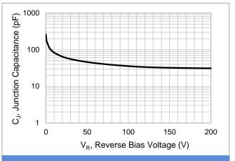
Fig.2 Typical Junction Capacitance
