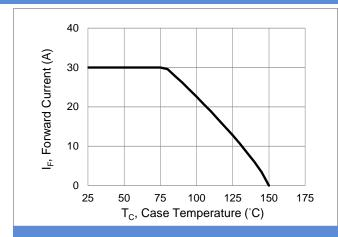
**Fig.1 Forward Current Derating Curve**
