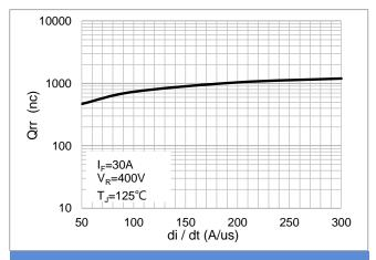
Fig.6 Typical Reverse Recovery Charges Versus di/dt
