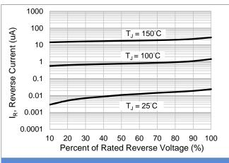
Fig.3 Typical Reverse Characteristics
