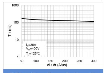
Fig.5 Typical Reverse Recovery Time Versus di/dt
