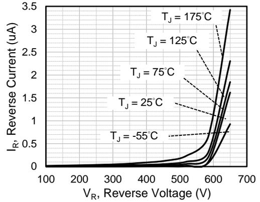
Fig.2 Reverse Characteristics
