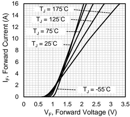
Fig.1 Forward Characteristics
