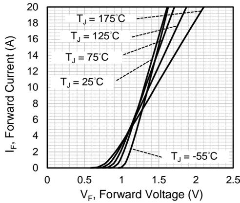
Fig.1 Forward Characteristics
