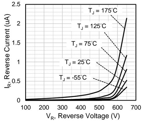
Fig.2 Reverse Characteristics
