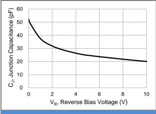
Fig.3 Typical Junction Capacitance
