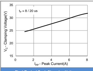
Fig.1 Typical Peak Clamping Voltage
