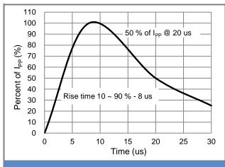
Fig.2 Pulse Waveform
